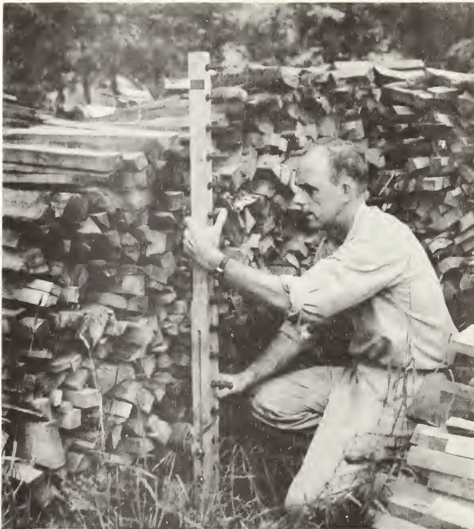
Figure 6.--Use of the special measuring stick for determining the percentages of wood and bark in a pile of slabs and edgings.
